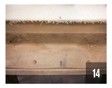
15. Remove c-clamps and come-a-longs. Work the liner down in the front corners, middle, and rear using the ratcheting cargo jacks, The longer the body, the more jacks will be needed. When the liner in the corners is less than 1" from touching the floor, install six to eight 3/8" x 2" elevator bolts with a lock washer and nut on each side of the doghouse. Use the spade bit to counter bore the plastic so elevator bolts are flush with the plastic.
